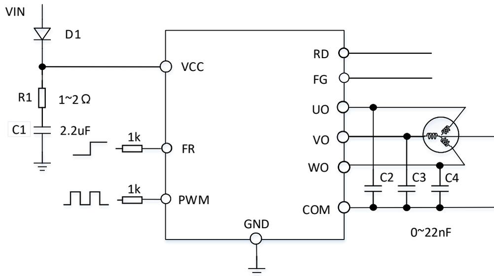
Note1: D1 is to prevent the damage from the power reverse connection.
