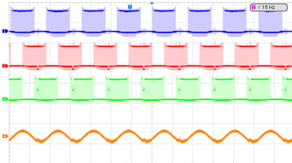
CH1:  $V_{u0}$ , 5V/div, DC ; CH2:  $V_{v0}$ , 5V/div, DC; CH3:  $V_{w0}$ , 5V/div, DC; CH4:  $I_{u0}$ , 200mA/div, DC
